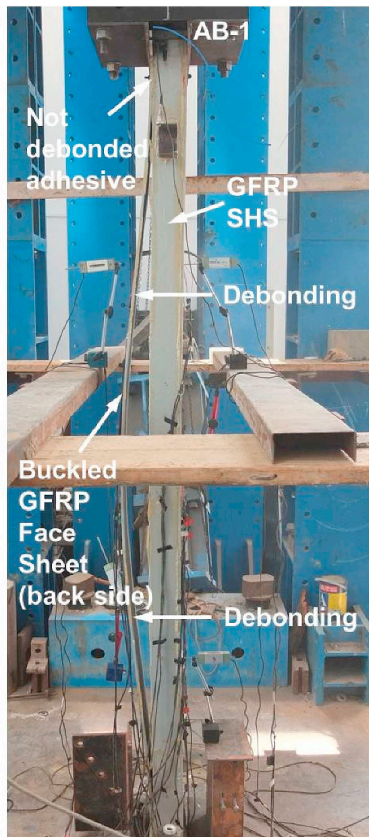
Fig. 5. Failure mode of specimen AB-1.
